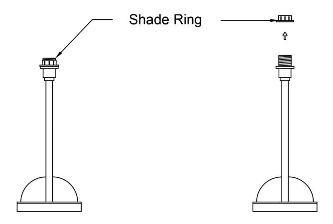
**STEP:-2** Place the shade on the bulb holder. Fit the shade ring back in position and tighten to rigidly fix the shade. Insert the bulb into the threaded socket.
