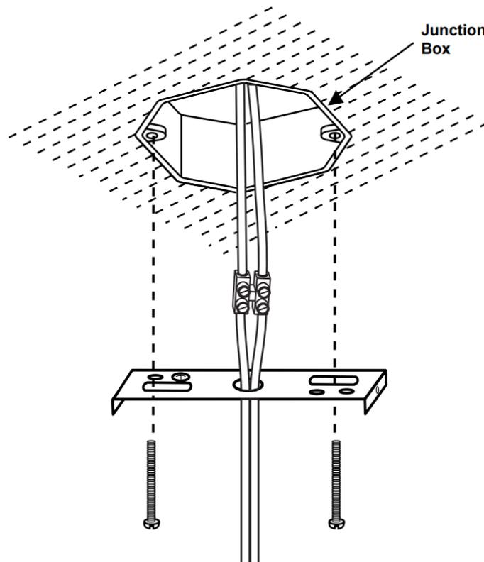
**STEP:-3** Place the ceiling cap over the bracket such that side holes are aligned of the ceiling cap & bracket. Insert the small screw into side holes and tighten with the screwdriver.
