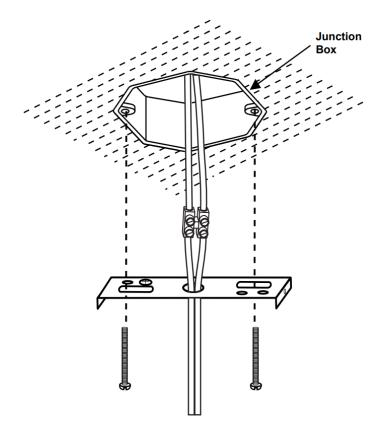
**STEP:-3** Place the ceiling cap over the bracket such that side holes are aligned of the ceiling cap & bracket. Insert the small screw into side holes and tighten with the screwdriver.
