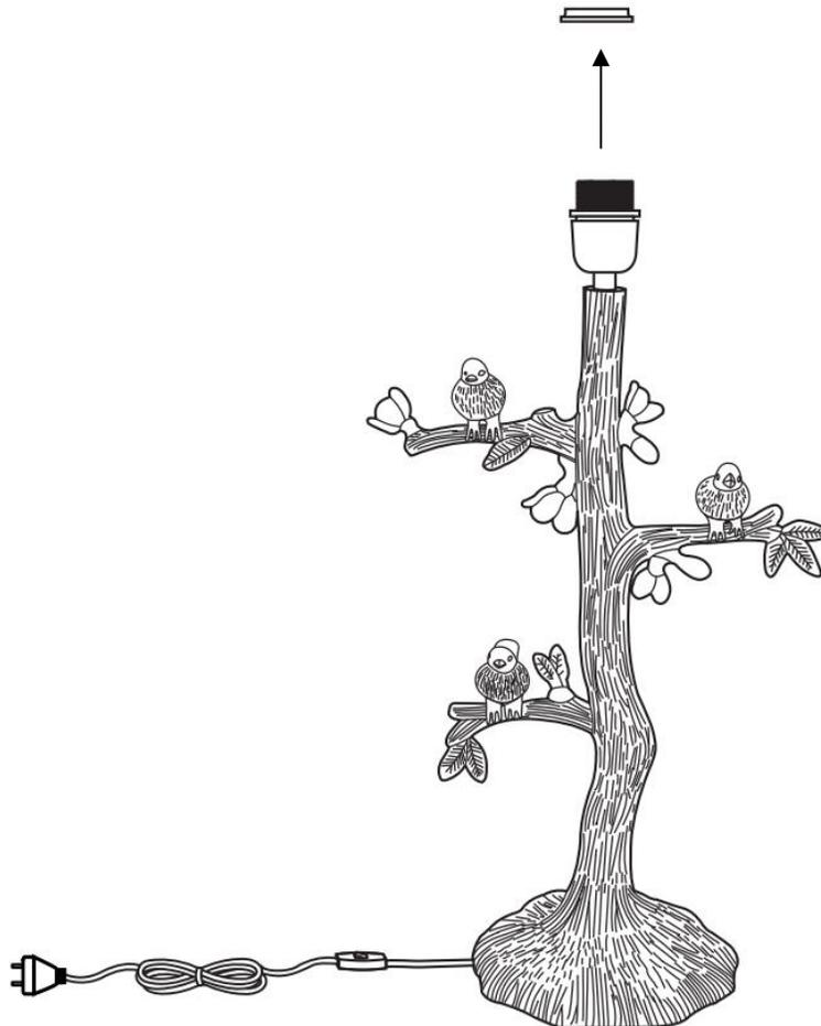
**STEP:-2** Place the lampshade on top of the light socket. Secure the lampshade by tightly screwing the Uno ring back into place.
