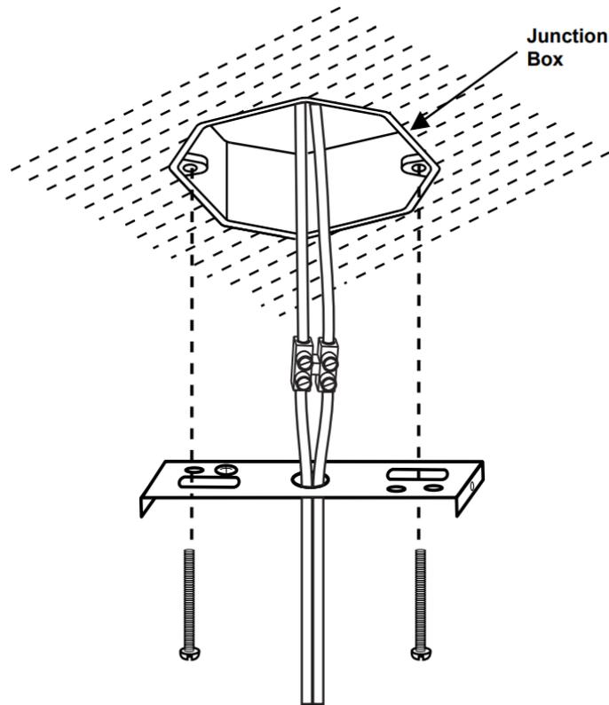
**STEP:-3** Place the ceiling cap over the bracket such that side holes are aligned of ceiling cap & bracket. Insert the small screw into side holes and tighten with the screwdriver.
