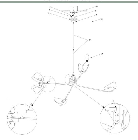
**STEP:-1** Attach the Crossbar(1) unto the junction box using the Mounting Screws(2). This fixture is designed to be mounted on standard round or octagon junction box. The junction box must be securely mounted to the structure of the building.
